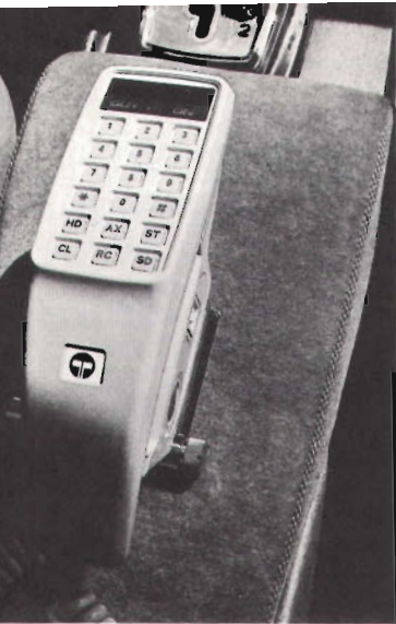
(Above left) Telecom's latest telephone equipment installed in a private car provides press button dialling for the subscriber.
